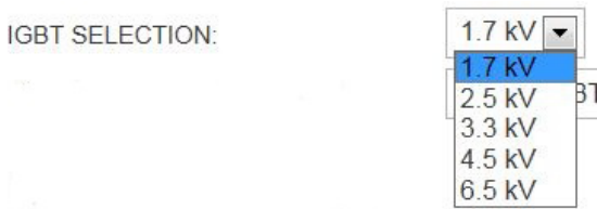
Figure 9. IGBT voltage rating input block
